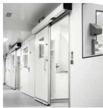
The hermetic sliding door from Gilgen automatically creates a seal for your rooms, preventing the unwanted exchange of air, impurities and other contaminants. When the door is closed, the pivot mechanism in the drive unit lowers the door leaf and presses it against the door frame. In combination with the sealing gaskets, this lowering movement ensures that the door creates a hermetic seal.
