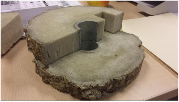
\*Cross cut Large Kit with a metal post, clearly showing the penetration into the ground
